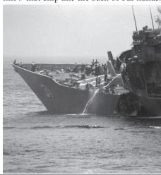
We send in our best firefighting teams and engineering teams to relieve the other crew. The first things that need to be done are to get the fires under control and dewater the ship. Dewatering is a process that gets the firefighting water out of the ship. The ship is listing heavily to port (the left side of the ship) and we've got to keep it from getting worse.
